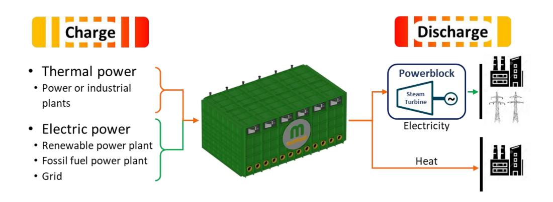
The charge / discharge of MGTES technology is focused on thermal storage by means of fluidized sand particles that allow to reach high temperatures with high diffusivity and reduced thermal losses.
